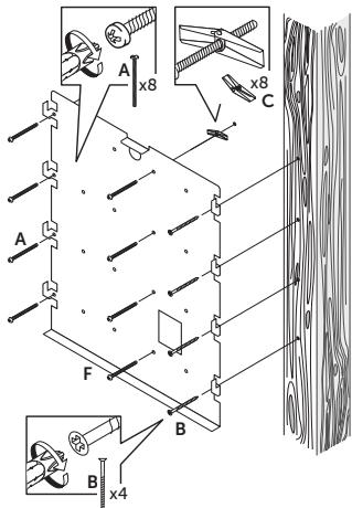
Important: Line up one row of holes along a stud in the wall and use the B screw.
