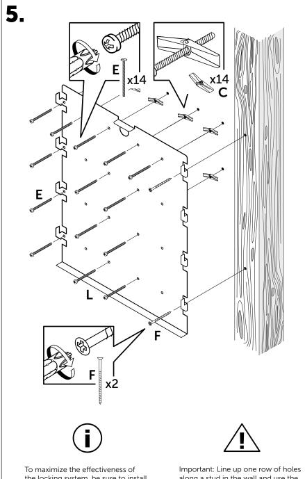
the locking system, be sure to install screws on bottom row and edges of the backplate. along a stud in the wall and use the F screw.
