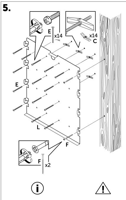
To maximize the effectiveness of the locking system, be sure to install screws on bottom row and edges of the backplate. Important: Line up one row of holes along a stud in the wall and use the F screw.
